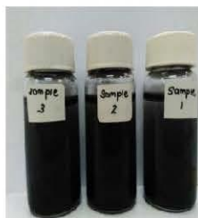
FIGURE 1. Graphene suspensions from samples prepared at different ball milling speeds for 30 min. (1) at speed 100 rpm, and (2) at 50 rpm. Pictures taken for composite samples dispersed in DW after 1 sonication
