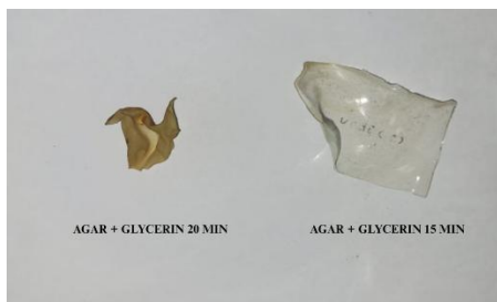
Fig. 4: Biodegradability Test Results of Biofilms Treated with Glycerin After One Week in Sand.
