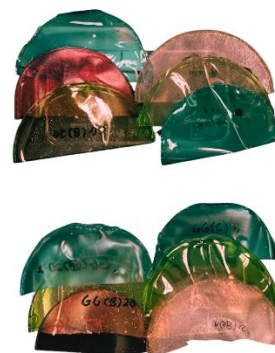
Fig. 2: Biodegradability Test Biofilm Before One Week in Soil and Sand
