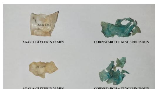
Fig. 3: Biodegradability Test Results of Biofilms Treated with Glycerin After One Week in Soil.
