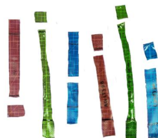
Fig. 8: Biofilm After Tensile Test.
